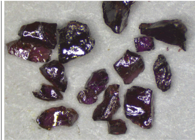
Pure LK-99 crystals made at a Max Planck Institute in Stuttgart, Germany.
